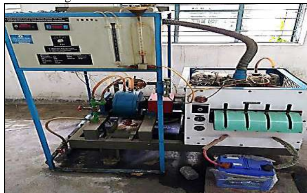
Fig 2 Experimental set up (ISUZU Engine)
