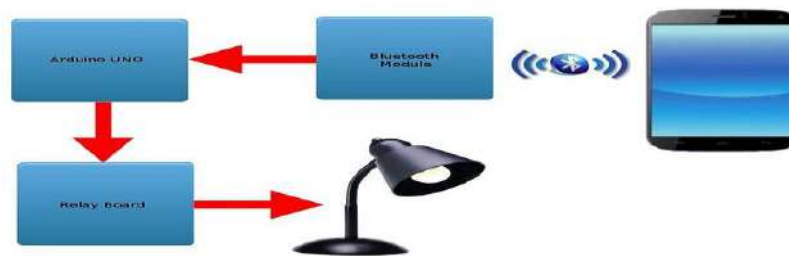
Figure: - 01 functional block diagram of home automation using Arduino Uno
