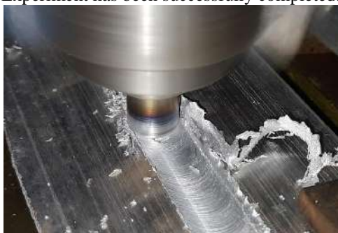
Fig 3.1: Friction Stir welding Process
