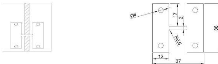
Fig-6 Dimension of specimen for tensile test
